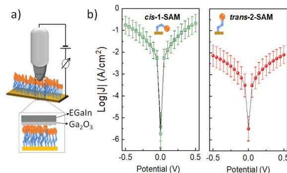
Fig. 4 (a) Scheme of the EGaIn/ $\text{Ga}_2\text{O}_3$ /*trans-1*-SAM/Au. (b)  $J/V$  plots acquired for *trans-1*-SAM and *cis-1*-SAM. Dots (circles and squares) indicate mean values while the bars stand for the standard deviation.
