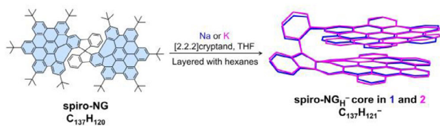
Scheme 1. Chemical reduction of spiro-NG with Na and K metals to afford the products 1 and 2 , cationic moieties and tert-butyl groups are omitted for structure clarity.
