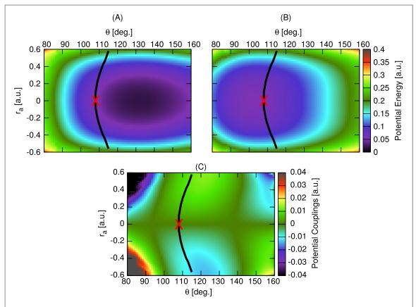
**Figure 2.** Two-dimensional diabatic potentials: (A) ground diabatic potential energy surface  $V_1^d$ , (B) excited diabatic potential energy surface  $V_2^d$ , (C) potential coupling surface  $V_{12}^d$ . The solid black line indicates the nuclear geometries at which the two diabatic PESs cross. The red cross indicates the CI geometry.
