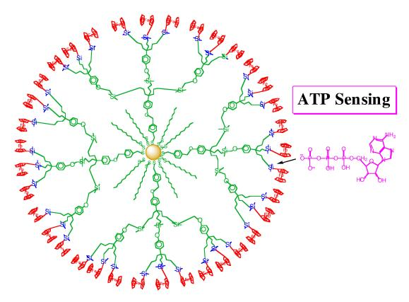
**Figure 3.** Redox ATP<sup>2-</sup> sensing using a large gold NP-cored silylferrocenyl-terminated *dentromer*. The cyclovoltammetry wave of the silylferrocenyl groups interacting with ATP<sup>2-</sup> is significantly shifted, allowing titration. Modified electrodes with this *dentromer* allow repetitive titrations.
