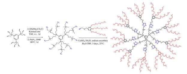
**Scheme 3.** Synthesis of the standard water-soluble *dentromer* terminated by Percec-type dendrons serving as micellar template for a variety of reactions catalyzed by transition-metal complexes or NPs in water or aqueous solvents.
