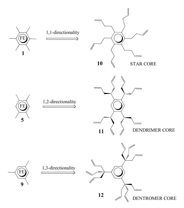
**Scheme 1.** Various directionalities quantitatively obtained upon perallylation of cationic polymethylbenzene iron sandwich complexes upon reaction with KOH and allylbromide in THF under ambient conditions followed by visible-light photodecomplexation. Complex  $\mathbf{1} = [CpFe^{II}(\eta^6-C_6Me_6)]$  [PF<sub>6</sub>]; in the scheme, FE =  $(\eta^5-C_5H_5Fe^{II})^+$  with the PF<sub>6</sub> counter anion.
