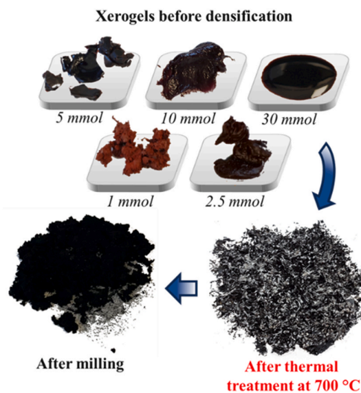
Fig. 1. Optical images of the xerogels prepared with different surfactant concentrations ( n_t = 1 –30 mmol), along with the resulting products from densification and agate-milling processes.
