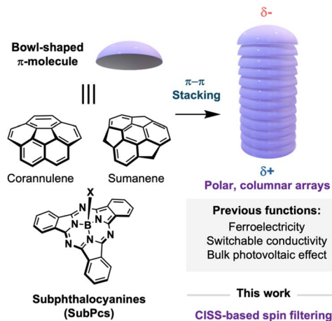
Fig. 1 Representative examples of bowl-shaped aromatics and a representation of their columnar self-assembly.
